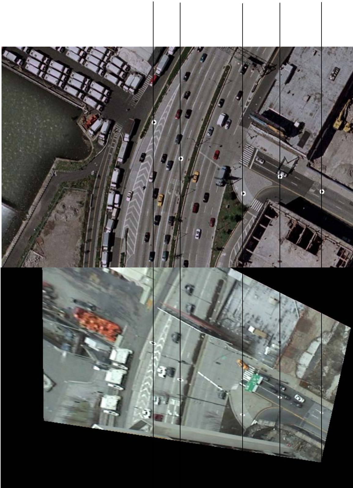
Figure 4 (Top) Overhead View with point correspondences. (Bottom) Side View projectively warped to overhead view, via computed Homography. Vertical lines are used to show accuracy of the mapping.
