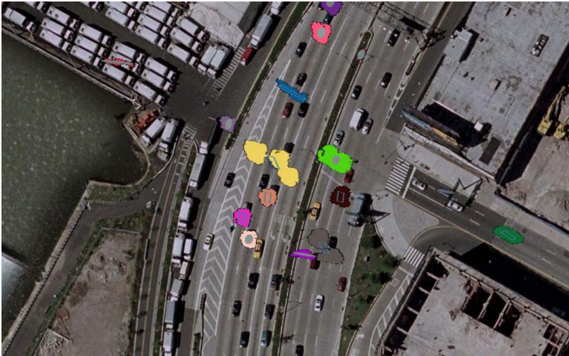
Figure 11: Example Overhead View depicting both the simple warping scenario where pixels C_1 are directly mapped to C_2 (colored blobs) and also the refined estimates of vehicle localization/orientation (grey ellipsoids/rectangles).
